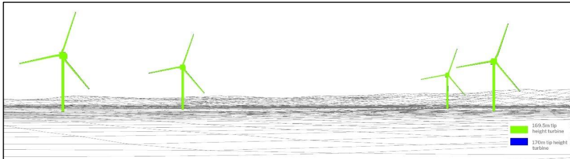
Figure 13-13: Turbine envelope comparison, where green indicates a 169.5m tip height option and blue indicates a 170m tip height option.
