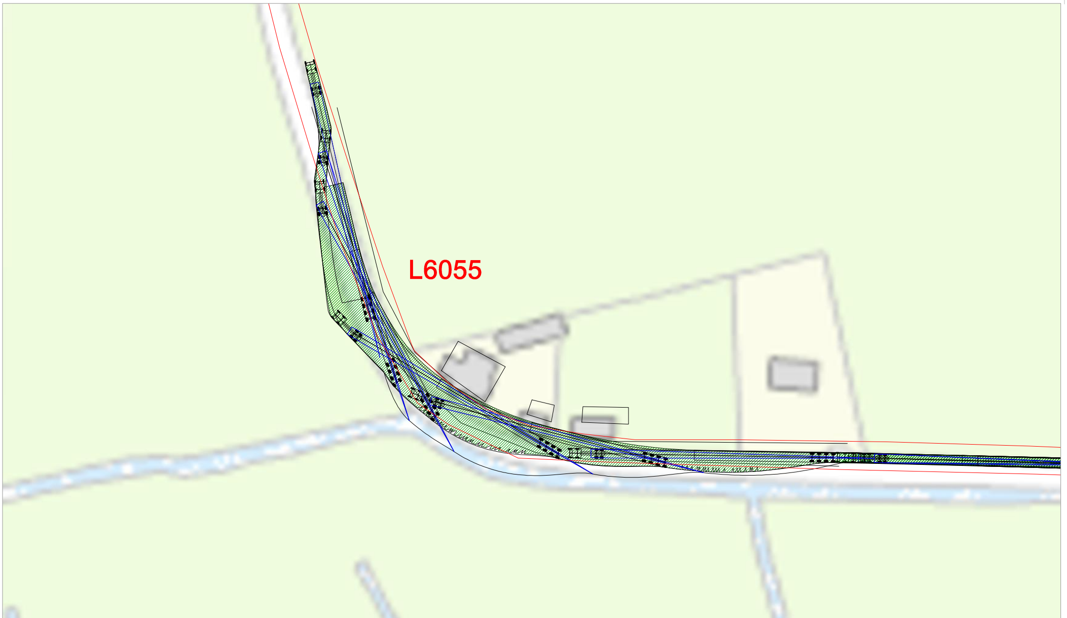
Figure 14-1-14 Location 5 - Bend on L6055, blade extended artic (73.65m blade)
