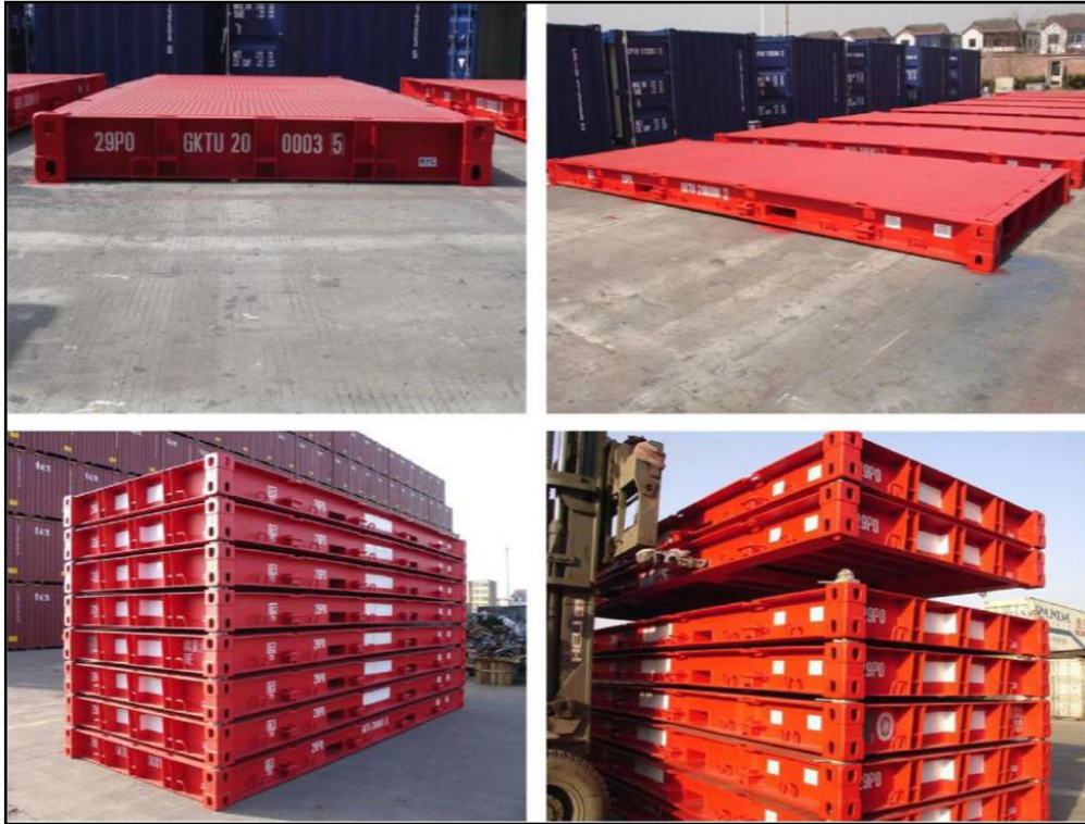
Plate 4.11 Flatracks for spreading load at laydown areas
