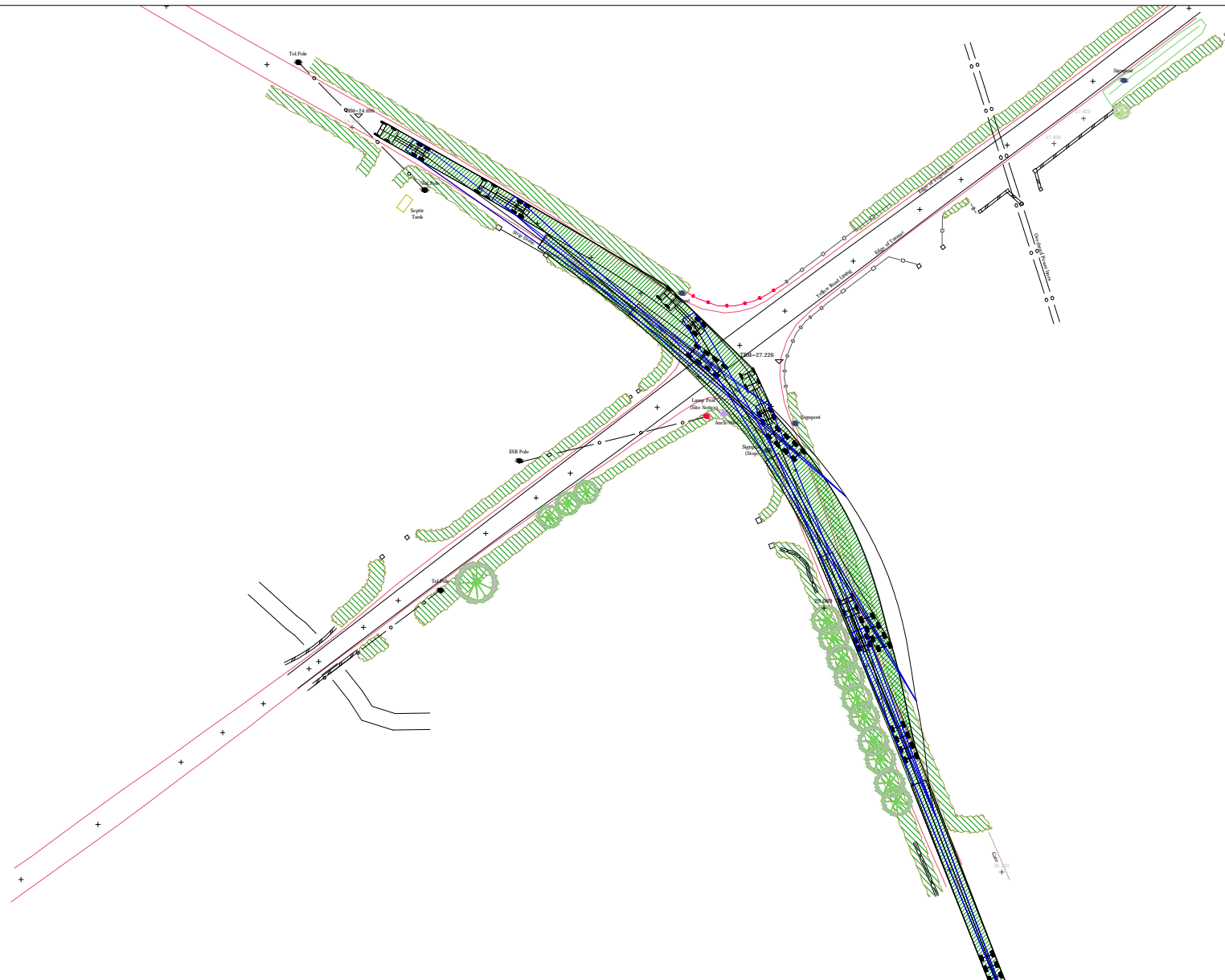
Figure 14-1-10 Location 3 - Crossroads on L6055 with L1027 - blade extended artic (73.65m)
