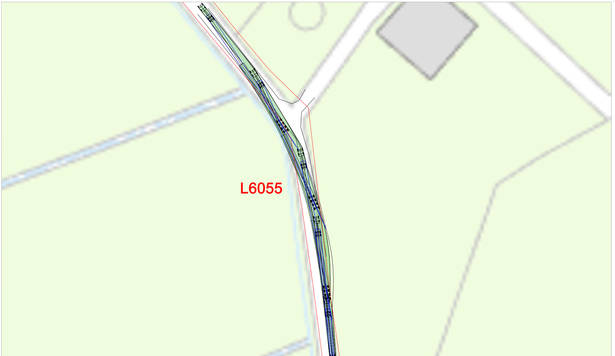
Figure 14-1-16 Location 6 - Bend on L6055, blade extended artic (73.65m blade)
